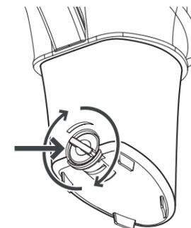
Then open the ceramic valve in the lower part of the attachment container so that the water can run through the filters.
