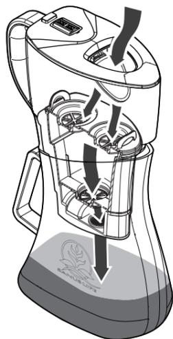
Then place the additional **ECAIA container S** (2-B) on the **ECAIA glass jug S** (2-A). As an alternative to the glass carafe, the tank container **ECAIA tank S** (2-C) can also be used. Note that the capacity of the tank is only 0.45 liters. Wait until all the water in the additional container has flowed through the filters into the glass carafe or tank container.
