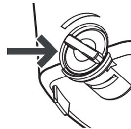
To regulate the ionization power even more precisely, you can also change the flow rate of the water. For this purpose, a ceramic valve is attached to the underside of the **ECAIA container S** (2-B) attachment container, which can be opened and closed. The more you close the ceramic valve, the slower the flow rate. Keep in mind: The slower the flow, the stronger the ionization.
